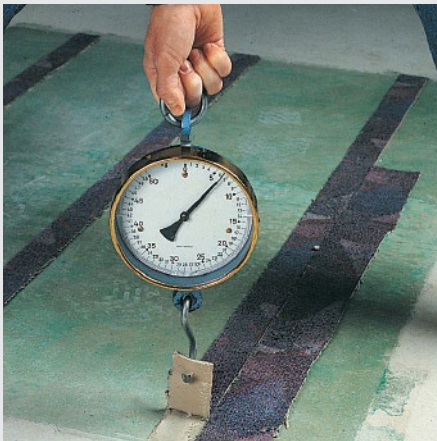
Bonding test and test of the resistance to peeling
