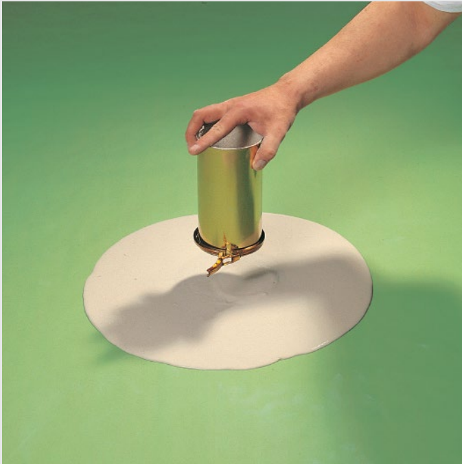
Determination of the slump-flow: Fill the consistency checking tin with mortar and lift it
