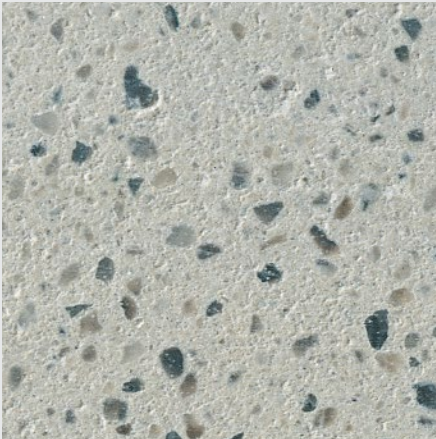
Knauf flowing screed cross-section, magnified by 4
