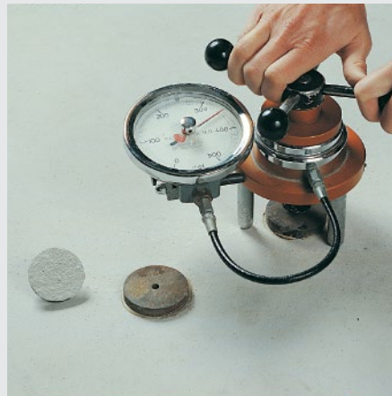
Test of the bond strength
