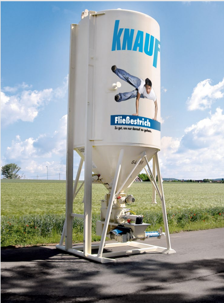
Knauf complete logistical service FERRO 100 with star wheel
